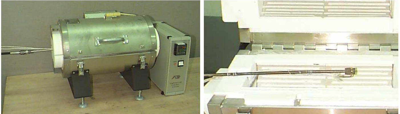
Figure 3.10.1 - 2, Thermal Cycle, Thermal Shock Test Configuration.
