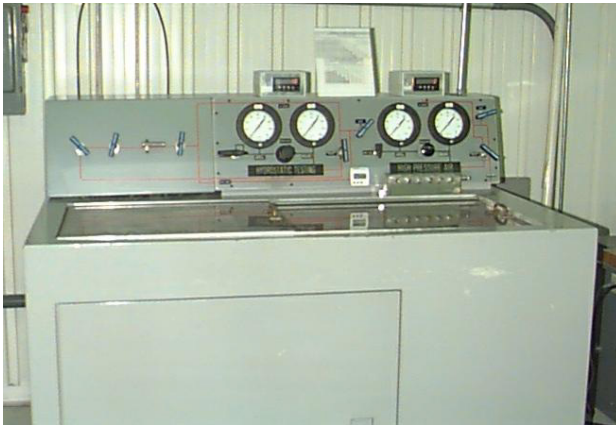
Figure 3.9.1 - 2, Gas Leak Test Configuration.
