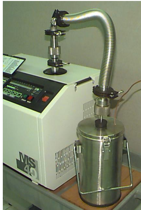
Figure 3.12.1, Low Temperature Helium Leak Test Configuration.
