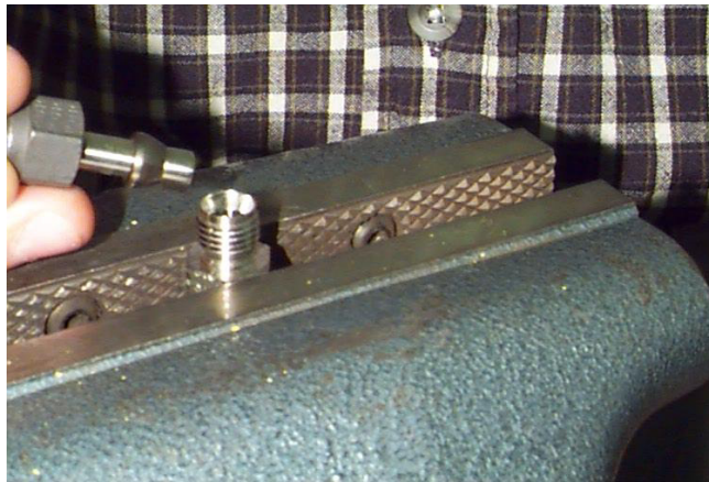
Figure 3.4.1, Repeated Remake Test (Size 8 Unilok)
