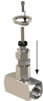
13. Slide the handle over the upper stem so that the threaded hole in the handle aligns with the set screw point on the upper stem. Insert the set screw into the handle's threaded hole and tighten with an allen wrench until "snug".
