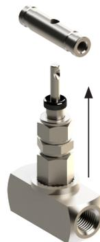
4. Loosen the socket set screw with an allen wrench and remove from the bonnet lock. The bonnet lock will now be free to lift up over the bonnet.
