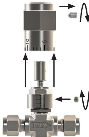
10. Place the handle on the stem so that the "zero" mark on the handle aligns with the "zero" mark on the barrel. Carefully tighten the set screw into the handle without losing the "zero" alignment.
