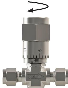
8. Move the micrometer barrel up under the handle so that the "zero" mark aligns with the bottom edge of the handle as shown. (The barrel may also be rotated to a position where measurements will be read from.) Then rotate the panel nut up against the barrel to temporarily hold it in place.
