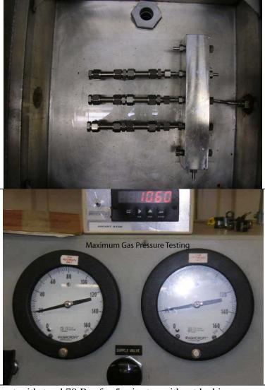
Comments: The samples must withstand 70 Bar for 5 minutes without leaking.
