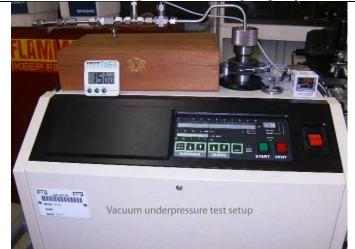
*Comments:* Subject test samples to negative 700 millibars for 15 minutes. Failure will be a rise in pressure of 30 millibars within 15 minutes.
