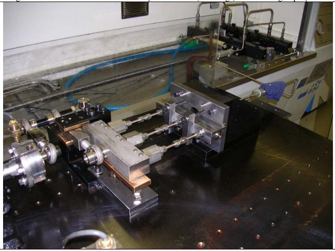
*Comments:* The samples must withstand planar vibration at the required stress levels of each size fitting for 20MM cycles, with simultaneous pressure impulse of 133% of working pressure for 0.5MM cycles without leaking.
