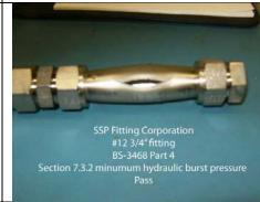
*Comments:* Choose an adequate tube gauge to ensure that test assemblies do not fail by premature bursting. Do not reuse these samples for other tests.
