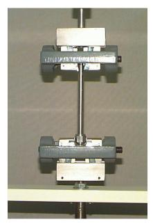
Figure 3.5.1, Tension Test Configuration.
