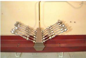
Figure 3.3.1 - 2, Hydraulic Impulse Test Stand and Fixture
