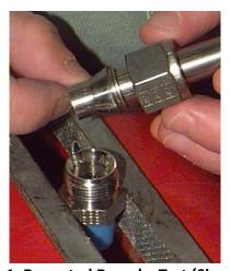
Figure 3.4.1, Repeated Remake Test (Size 8 Duolok)
