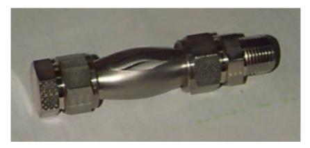
Figure 3.2.3, Burst Test Specimen
