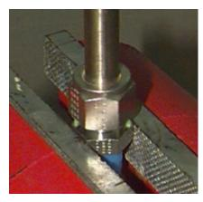
Figure 2.1.2 Initial Makeup: Fitting Assembly
