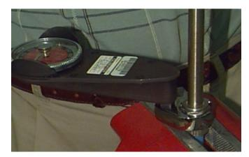
Figure 2.1.1 Initial Makeup: Torque Measurement
