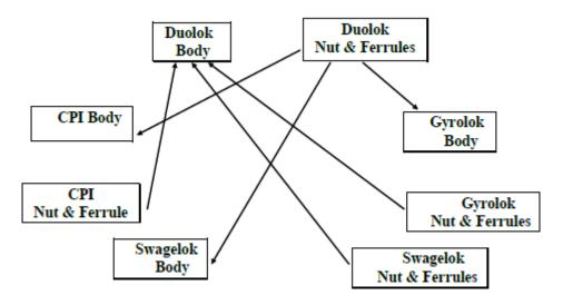
Figure 3.8.1, Interchange Test Combinations
