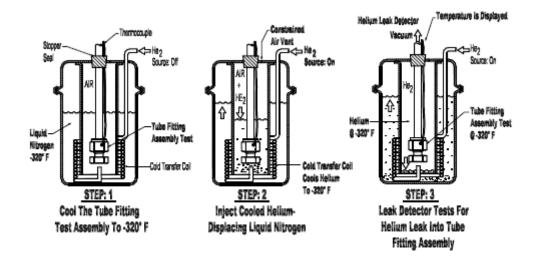
Figure 3.12.2, Low Temperature Helium Leak Test Sequence.
